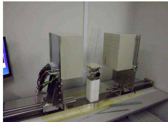
Fig 1:Beam ON-LINE PET System
